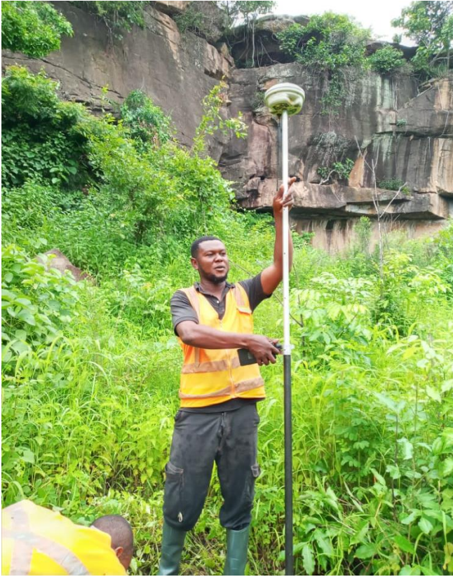
Caption: Ground control set-up
