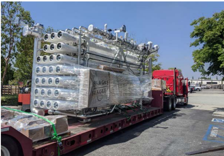
Caption: Partial shipment of the Perris II Desalter 3-stage reverse osmosis system
